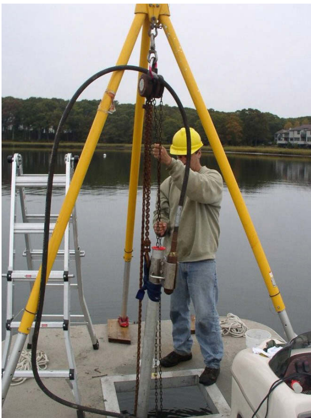
Figure 4.—A vibracore used to sample subaqueous soils.
