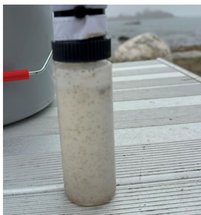
Example of when to cut the tip of your pipette – this sample has many “large” zooplankton that you may not capture otherwise
