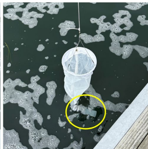
Ensure the collection bottle (secured to the mouth of the plankton net) is filled with water before towing the net; this helps to ensure the net will stay submerged during the tow
