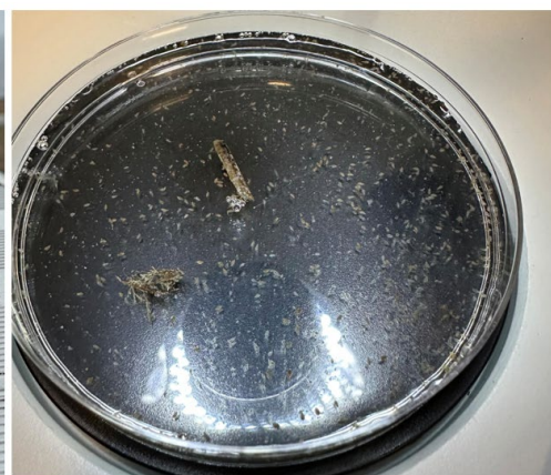
Example of when to cut the tip of your pipette – this sample has many “large” zooplankton that you may not capture otherwise
