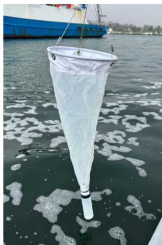
Ensure the collection bottle (secured to the mouth of the plankton net) is filled with water before towing the net; this helps to ensure the net will stay submerged during the tow
