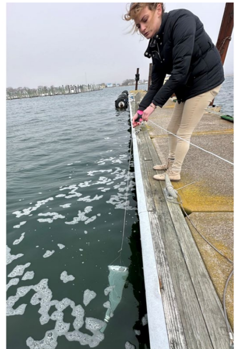
Maintaining a consistent speed and for a predetermined duration, tow the submerged net at the desired depth
