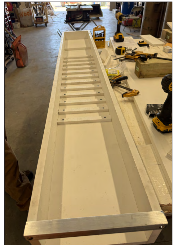
Figure 11. A prototype eelgrass sluice that will be tested by CCE and UConn in 2026.
